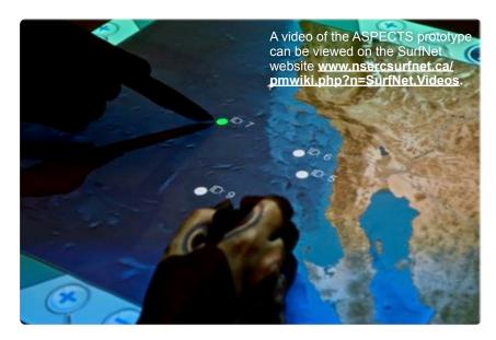
ASPECTS users can view, manipulate, and share dynamically updated map-based information in a windowing environment optimized for tabletop systems. The system provides the ability to easily rotate, move, and resize windows, as well as access system menus from anywhere around the table. ASPECTS is designed to run on an Anoto digital pen tabletop hardware platform, that provides unique user
